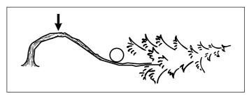
Decide which is the SAFEST way to release the tension and whether YOU are able to do it safely. In complicated situations the only safe method is to put aside your chain saw and use a winch.
